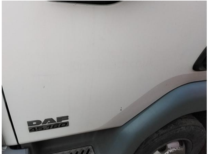
4: Door nsf Chipped Multiple Chips
